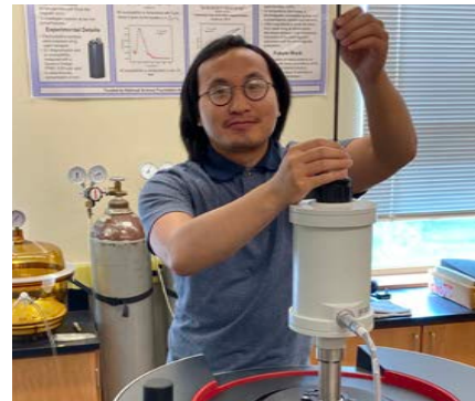
Young Moua inserting a sample in the DynaCool Physical Property Measurement System in Paul Shand's research lab.
